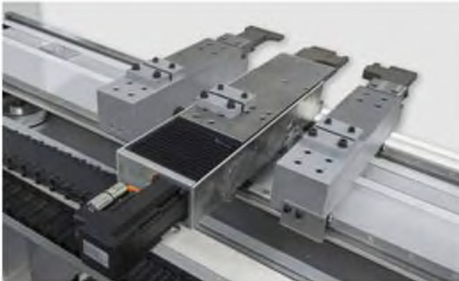
Additional backgauge finger for gauging long parts
