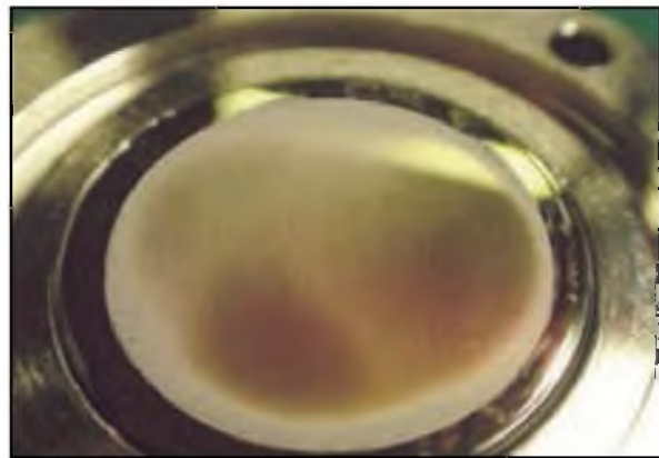
The resonator mirror without a centrifugal separator To prove the efficiency of the cyclone cleaner unit, the laser gas was contaminated with 5 gr. of glass powder
