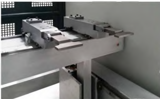
Standard two-axis backgauge (X, R) with manual Z-axis on PPEB-4 and PPEB-5
