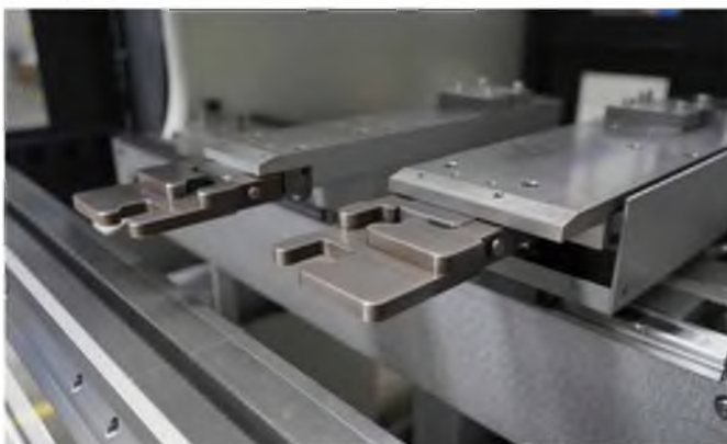
Five-axis backgauge (X, R, Z1, Z2, X') on PPEB-8
