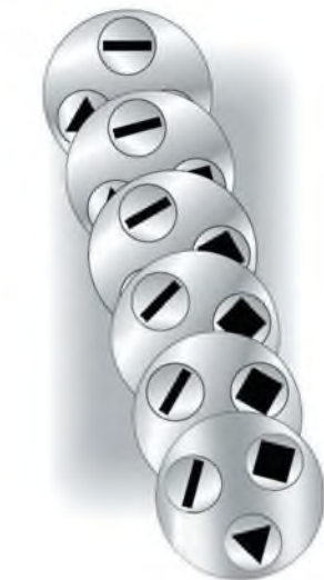
The Multi-Tool indexing mechanism allows any selected punch to be oriented in increments of 0,01° to any programmed angle automatically.
