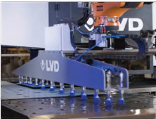
Pick-Sort system loads full size sheets and automatically retrieves and stacks individual punched parts.
