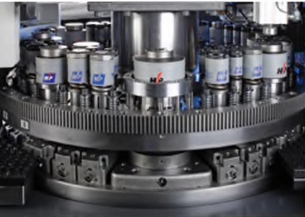
A large capacity turret features 48 stations.
